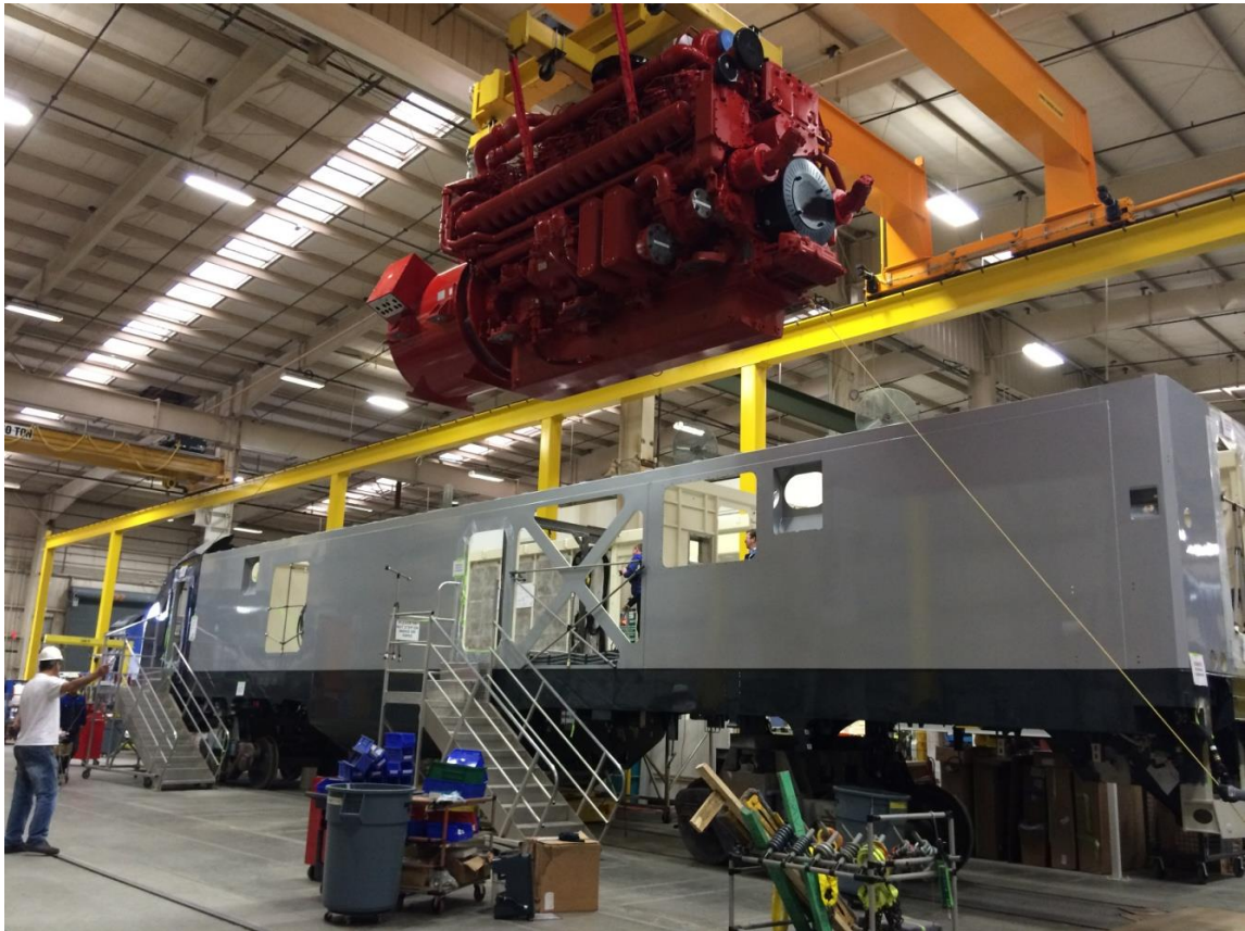
Charger Locomotive Production Diesel Engine installation
