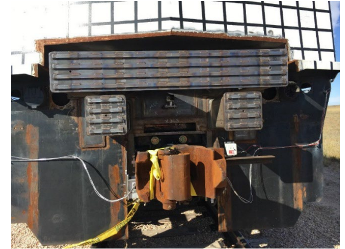
CEM system retrofit onto existing locomotive
